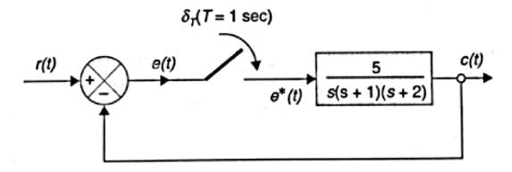
15. Determine the pulse transfer function and stability for the following system using Bilinear transformation. (Given transfer function of  $ZOH=(1-e^{-Ts})/s$ )
