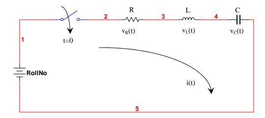
When switch is closed at t=0, apply KVL
